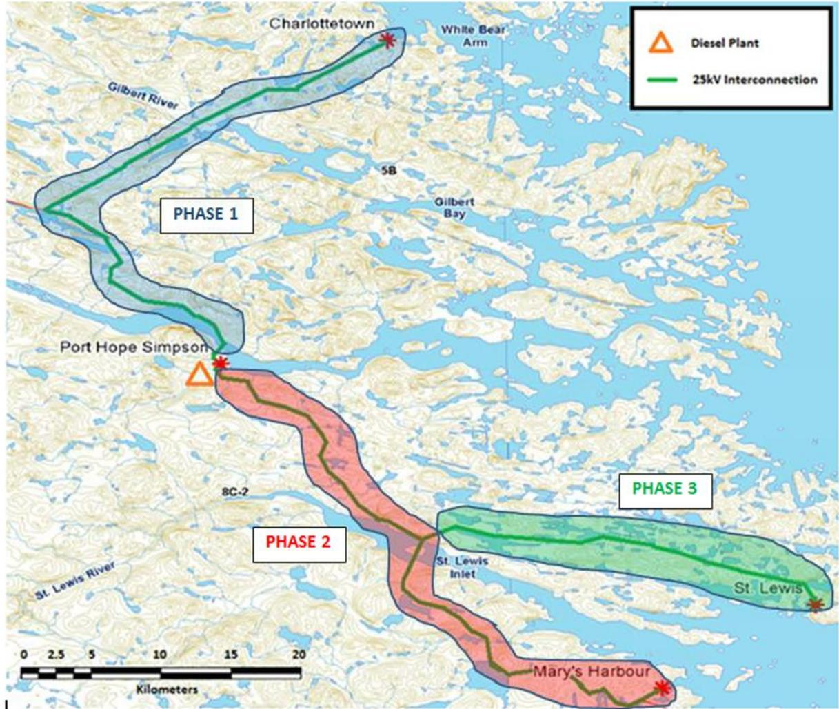
Figure 3: Alternative 3a: Southern Labrador Interconnection – Phased Approach
