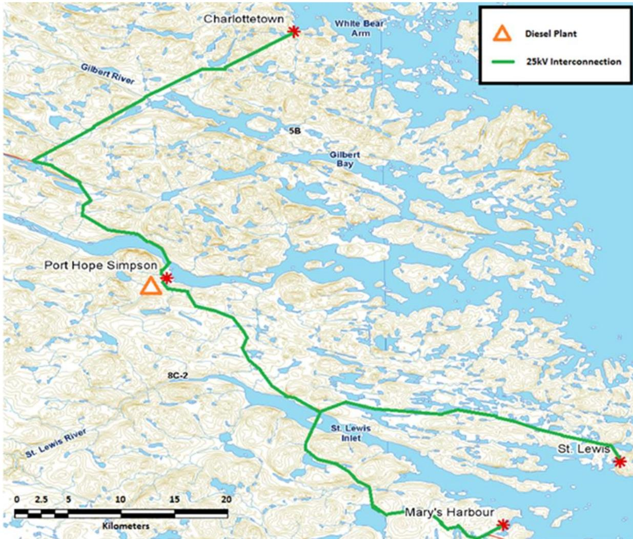
Figure 7: Southern Labrador Interconnection – Full Interconnection
