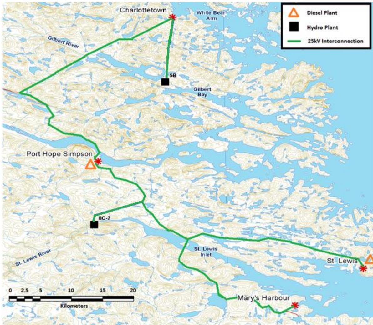
Figure 2: 25 kV Interconnection – Hydro Option
